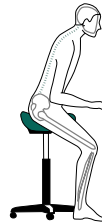
Spinal position leaning forward on Saddle Seat; action takes place at hips.
